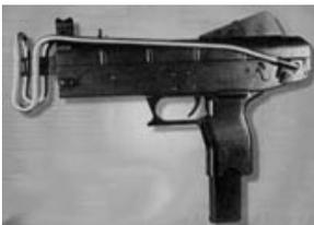
This SMG was constructed to decide most widespread SMG`s problems - rate of fire not lower than 450-600 shots per minute and avoiding large dispersion. To make it real the inventors created the "dynamic deceleration" system. In this reason "Baksan" uses only SP-10 (9x21 mm), SP-21 SMG, and 9mm PM bullets. SP bullets: 20 in magazine, 6in burst. 9mm PM: 30 in magazine, 10 in burst.
