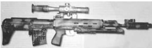
This sniper rifle was invented by the initiative of "Vimpel" ("The Pennon") special team and was accepted by all of the Russian special forces. This SVD replace also uses 7.62mm ammo. With 20-shots magazine it has an automatic mode (6 shots in burst). You
